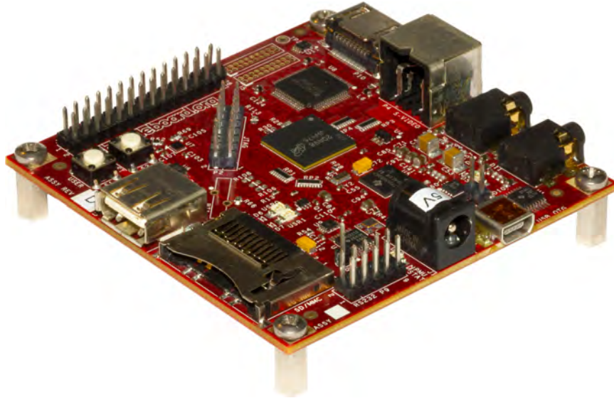
Figure 3.2: The Texas Instruments OMAP3-based BeagleBoard
